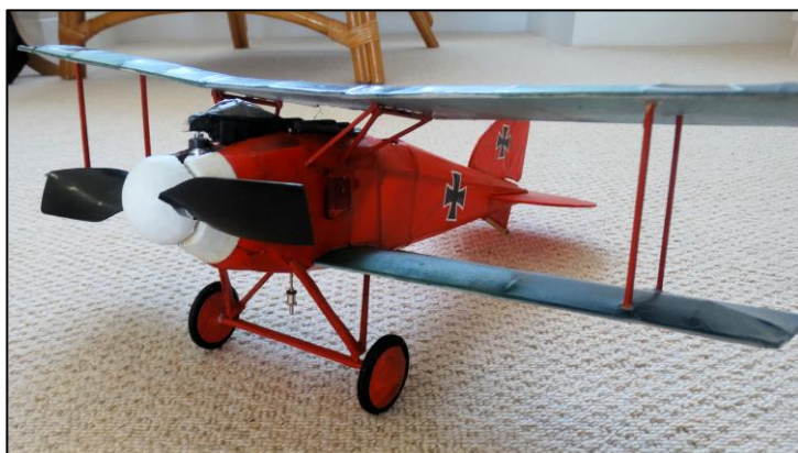
Motor fairly well concealed, that may or may not be such a good idea. Spinner plunge moulded from celluloid. This will be glued to the ply backplate once access to the motor mounting screws to adjust down/side thrust is no longer required. Total weight 51.2gms including Basswood struts and wire in the front undercarriage struts. Colour scheme is that of Karl Allmenruder of Jasta 11.
